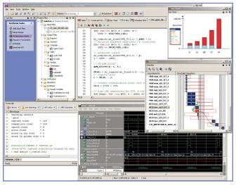
Catapult integrates a fully automated verification flow, including linting and code coverage of the input source code and push-button simulation of the generated RTL, for higher quality results.
