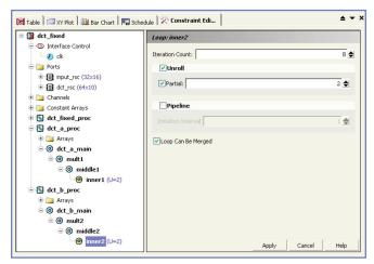
Optimize hardware by applying architectural constraints to unroll, merge, and pipeline loops, map arrays to RAM, and control resource allocation.
