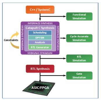
The Catapult design flow enables the evaluation of a wider range of micro-architectures than possible using hand-coded methods.
